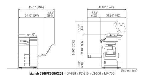
NOTICE: Be sure to allow a clearance of 8 inches (200 mm) or more at the back of this machine for the ventilation duct.
